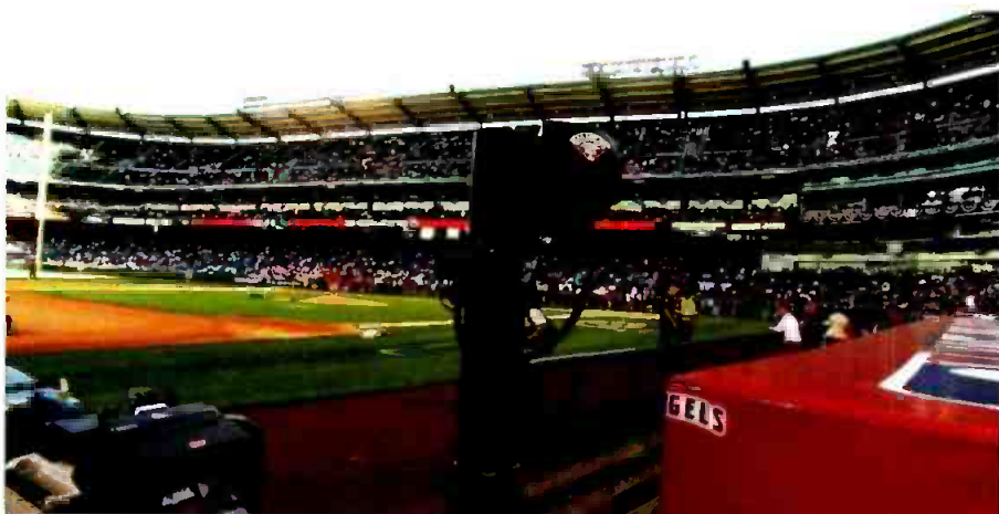
The dugout cameras, used for capturing field and stadium views, are each mounted to a Telemetrics Televator EP-S3 weatherproof elevating pedestal. Image courtesy MLB Network.
